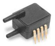
ASDX Series pressure sensor, amplified, differential/gage, 0 psi to 5 psi operating pressure, "D4" DIP package, straight port
